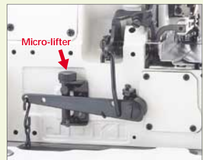
Bottom and top differential-feed micro adjustment mechanism
