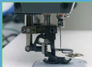
Top feed presser foot mechanism
